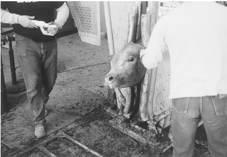
Figure 8.9. Steer held in a squeeze chute with a curved bar headgate. This type of headgate provides good control of head movement and it must be used with a body squeeze to prevent the animal from lying down. If the animal lies down, it can choke. If a headgate is used with no body restraint, it should have straight vertical neck bars that allow the animal to safely lie down with no pressure on the underside of the neck. These principles apply to all species.
